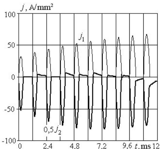
Fig. 3. Electromechanical characteristics of the IDC when excited by a packet of pulses from the CES sections of the same capacitance  $C_0 = 100 \mu\text{F}$ , charged to different voltages  $U_0$
