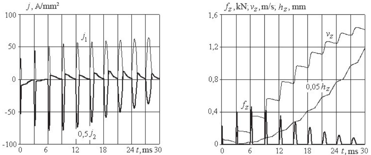
Fig. 4. Electromechanical characteristics of the IDC when excited by a packet of pulses with a period of 3 ms, from the CES sections charged to a voltage  $U_0 = 210$  V, which capacity  $C_0$  increases linearly
