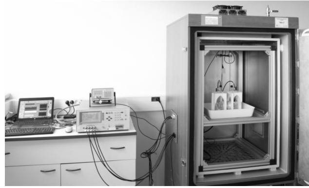
Fig. 2. Overall view of the configuration of the national measurement standard of electrolytic conductivity
