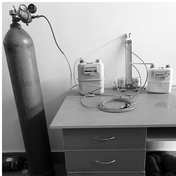
Fig. 1. Experimental model of a prototype test system for the tightness of gas meters under the action of hydrogen gas
