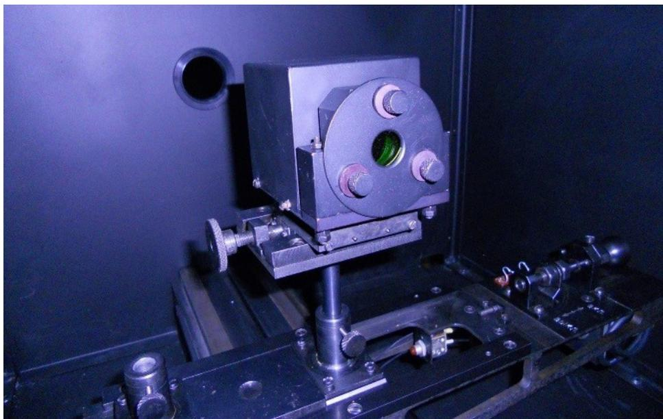
Fig. 4. Standard photometer based on trap detector with  $V(\lambda)$  corrective filter
