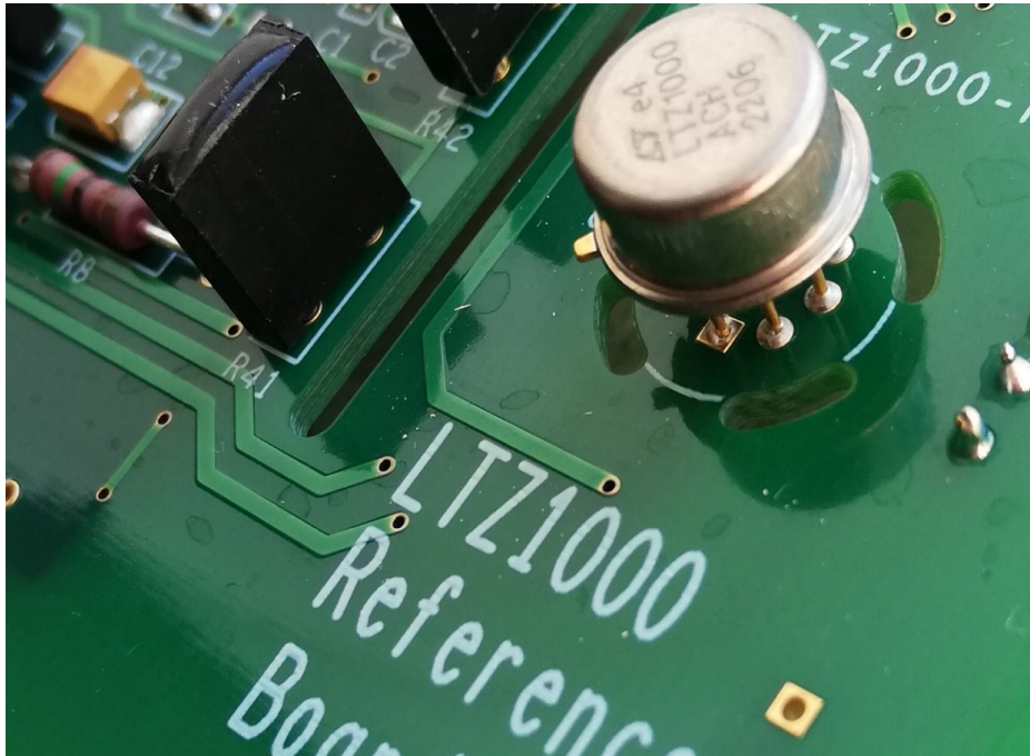
Fig. 2. Exterior view of the LTZ1000 integrated circuit [7]
