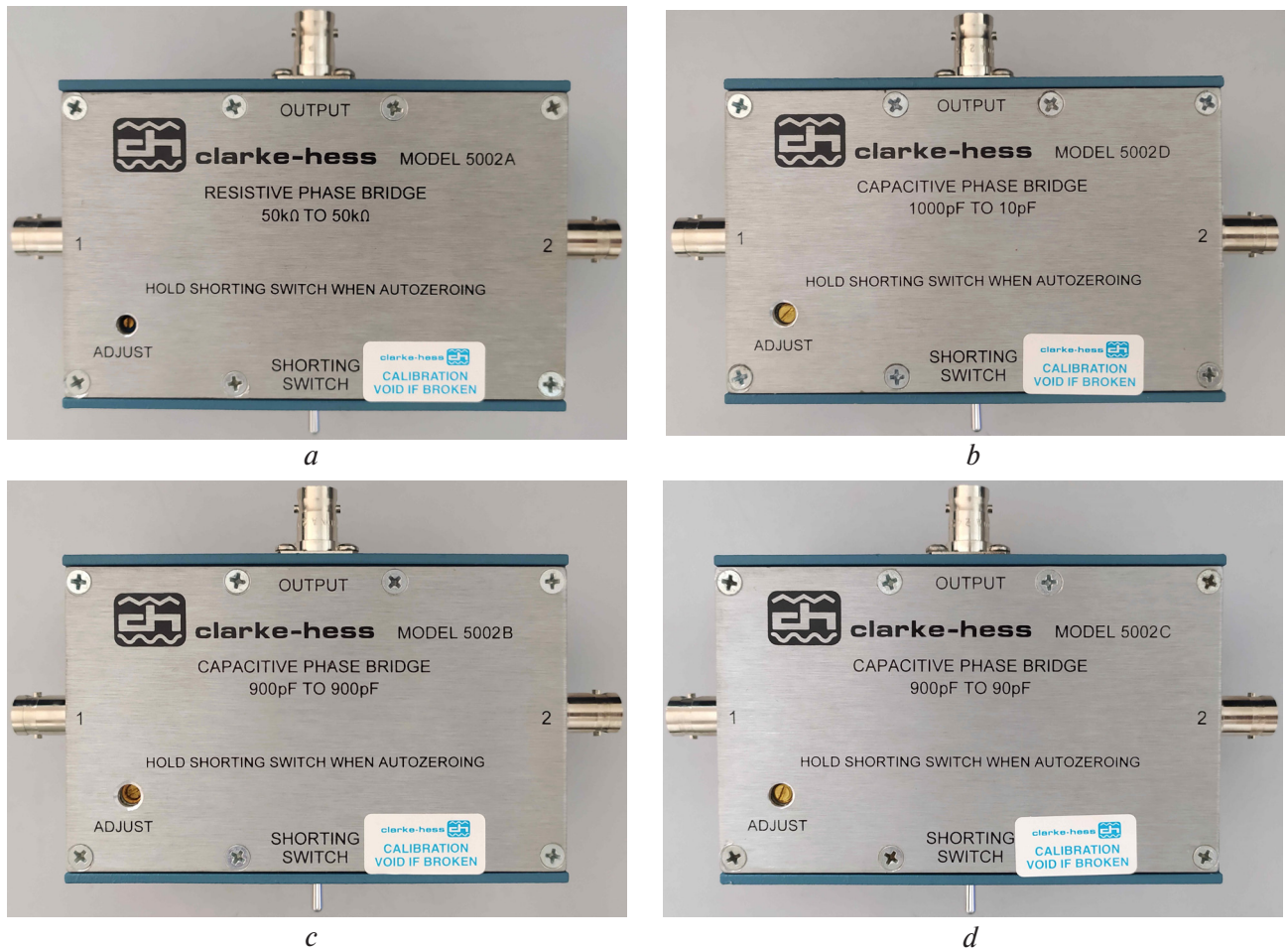
Fig. 3. Resistive and capacitive phase bridges: a – 1:1R; b – 1:1C; c – 10:1C; d – 1000:1C
