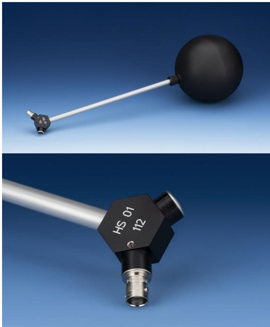
Fig. 1. Seibersdorf HS01 reference chamber for H^*(10) (Photo: Bildstelle PTB)
