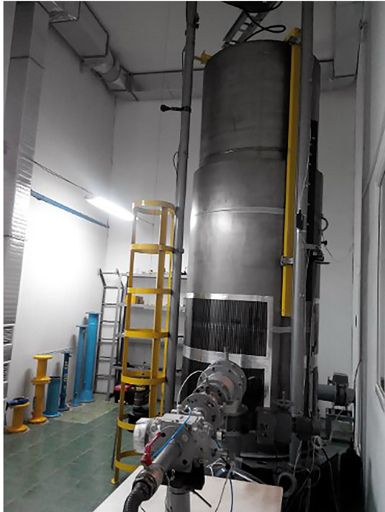
Fig. 2. State primary measurement standard of units of gas volume and volumetric flow rate (CMC-entry – UA1) – DETU 03-01-15
