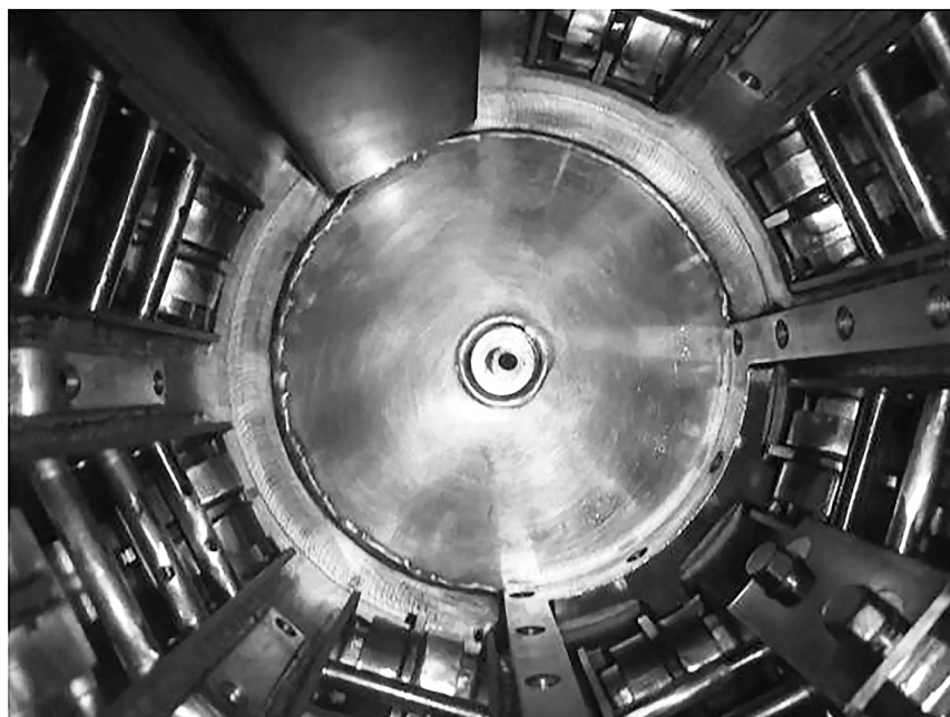
Fig. 4. Magnetic discharge ion-heterodyne pump of Ch1-70 time and frequency measure consisting of 7 open and one closed cell
