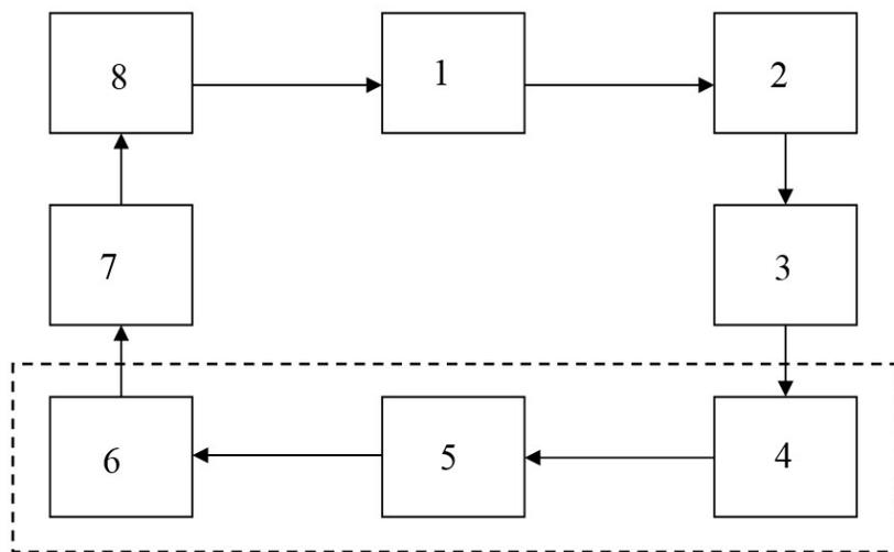
Fig. 2. Block diagram of the experimental setup for recording the output voltage of pyroelectric converters: 1 – personal computer (PC); 2 – DAC; 3 – radiation source driver; 4 – IR emitter; 5 – optical matching device; 6 – pyroelectric detector; 7 – pyroelectric detector driver; 8 – ADC
