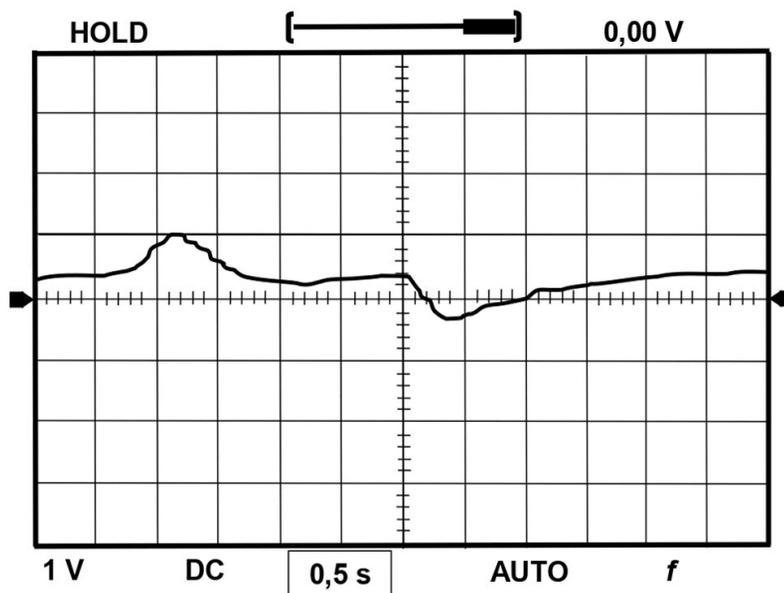
Fig. 3. Oscillogram of the pyroelectric response of a Z55 detector to the stepwise switching on the IR source
