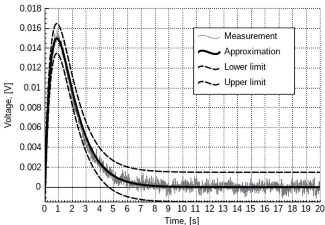
Fig. 4. Experimental (noisy) and normalized model (solid) time dependencies of the pyroelectric detector LHI958 with approximation parameters: smaller time constant 0.6 s, larger time constant 1.3 s, normalizing coefficient of the amplitude of the approximation curve  $K=0.054$  V
