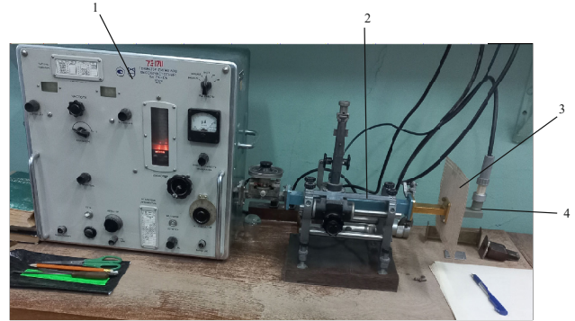
Fig. 10. Experimental setup (9–12 GHz) 1 – generator, 2 – measurement line, 3 – screen, 4 – detector section
