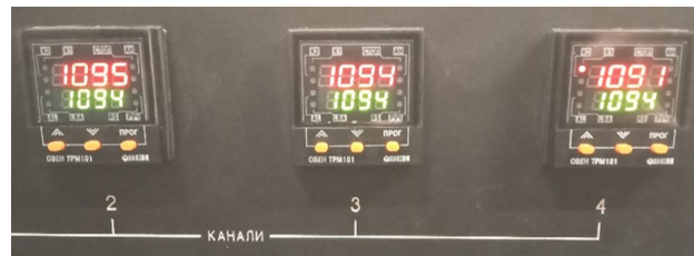
Fig. 6. Process of the “Promin-V/1350” radiator temperature reaching the 1094 °C regime
