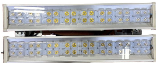
Fig. 2. Modularity of the luminaire due to increased power
